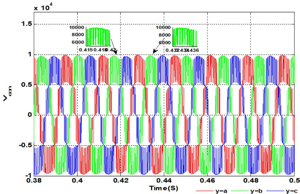
Figure. 8 MMC output voltage for sorting algorithm
