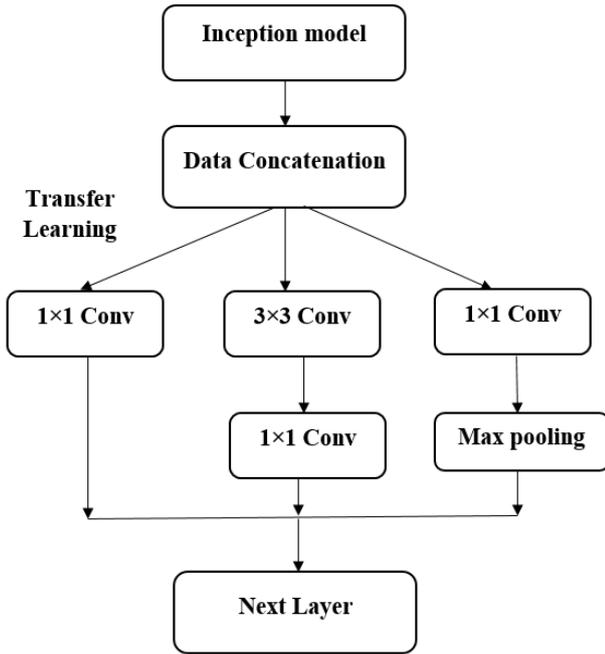
Figure.2 Inception model’s working procedure
