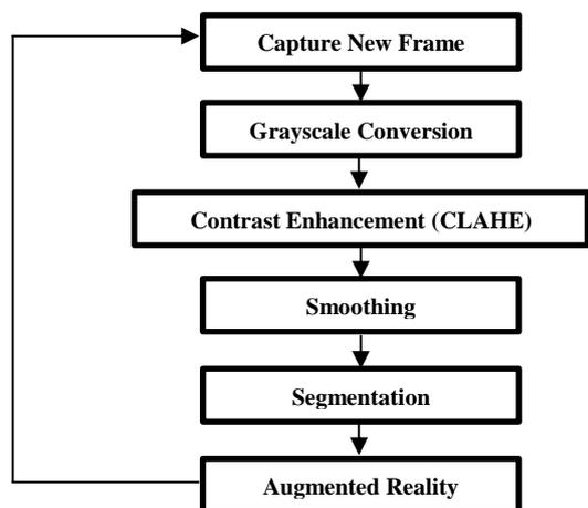
Figure. 3 Real-time vein mapping system diagram
