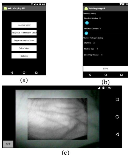
Figure. 6 Screenshots of the prototype android app: (a) main screen (b) setting screen, (d) view screen
