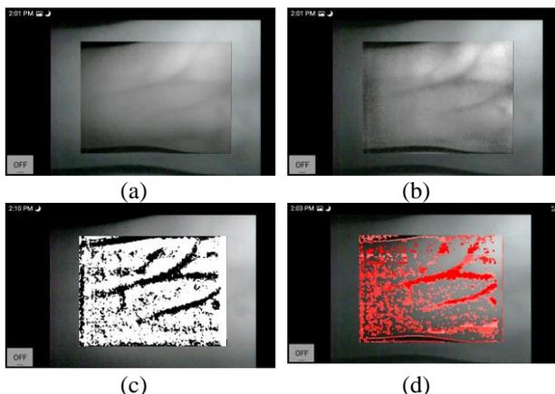
Figure 7. Sample results for a wrist: (a) grayscale frame (b) applying contrast enhancement CLAHE (c) adaptive thresholding, and (d) color veins
