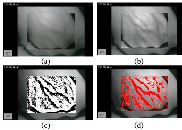
Figure 8. Sample results for a dorsal hand: (a) grayscale frame (b) after applying contrast enhancement CLAHE (c) adaptive thresholding, and (d) color veins
