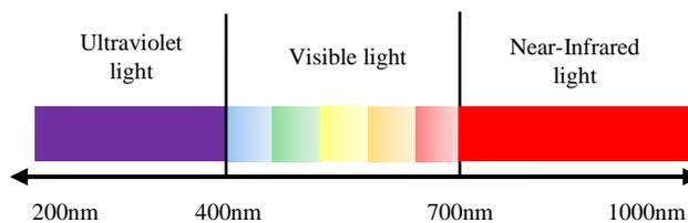
Figure. 1 The wavelength of near-infrared light
