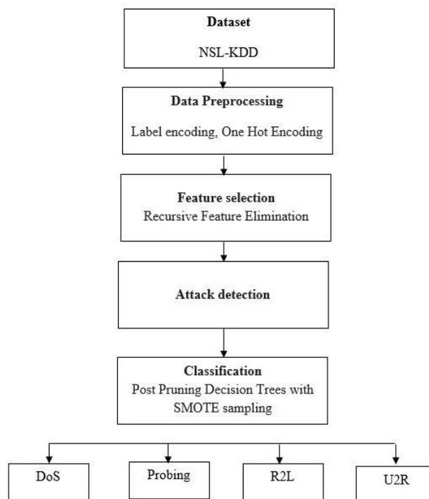
Figure. 1 Block diagram of the proposed PPDT-SMOTE technique
