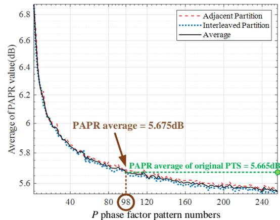
Figure. 3 Optimization of phase factor pattern numbers for proposed scheme with  $W=4$  and  $V=4$
