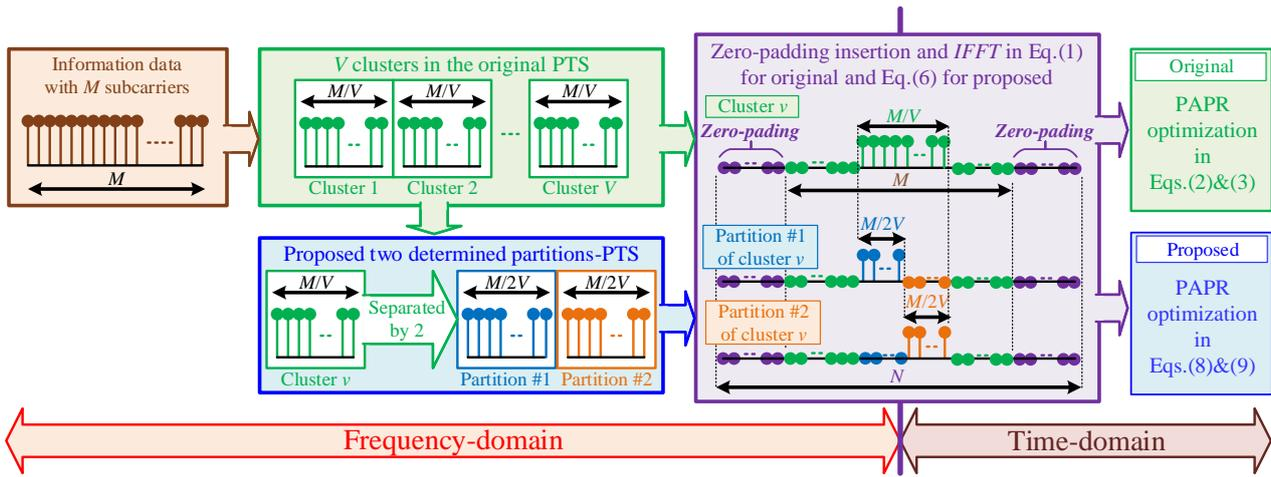
Figure. 1 Two-partitioned concept in the proposed PAPR reduction
