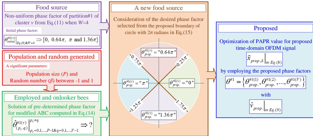
Figure. 2 The proposed phase factors generated by the modified ABC technique
