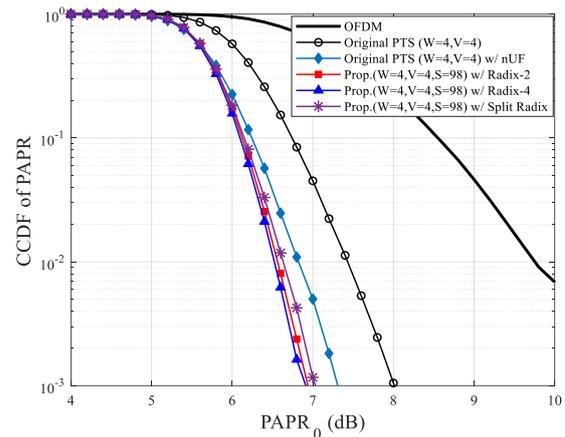
Figure. 5 CCDF of PAPR for interleaved
