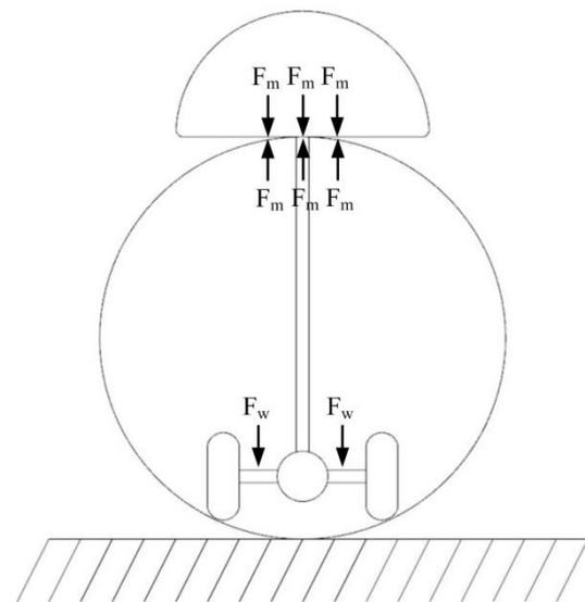
Figure. 2 Diagram illustrating the forces inside the spherical magnetic robot
