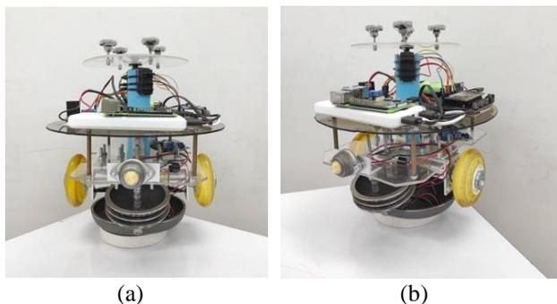
Figure. 6 A schematic view of proposed CE-R1 spherical magnetic robot: (a) front view and (b) side view
