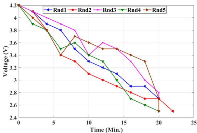
Figure. 12 Five random tests of CE-R1 robot power supply with the different routes
