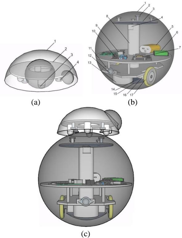
Figure. 5 Head and body of CE-R1 robot design: (a) head (b) body and (c) structure inside of CE-R1
