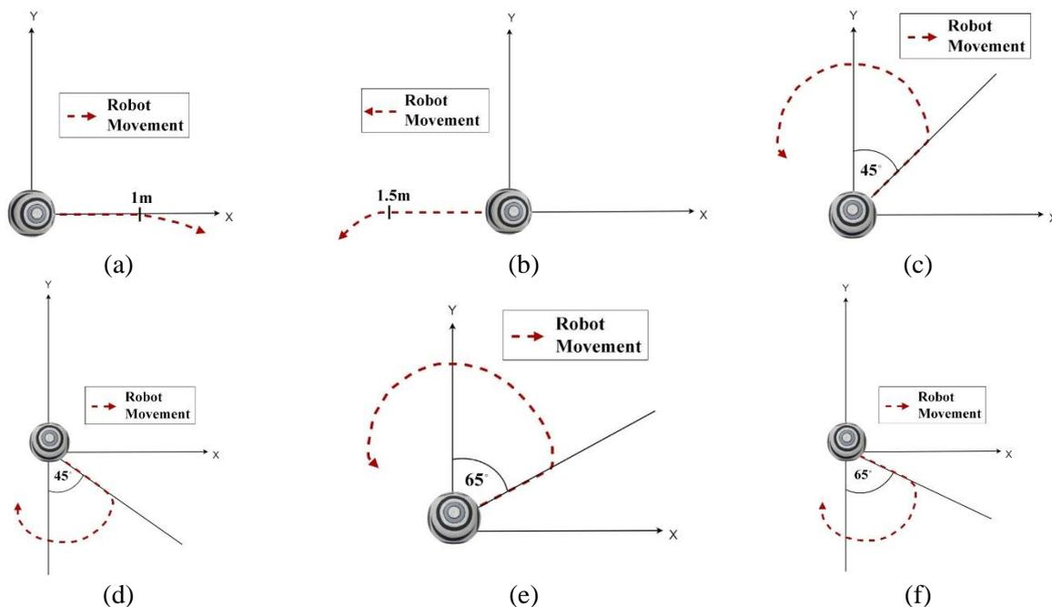
Figure. 11 Spherical magnetic robot CE-R1 movements at a top view: (a) forward (b) backward (c) turn left (d) turn right (e) turn left 65 degree and (f) turn right 65 degree
