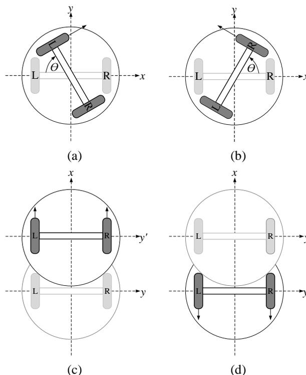
Figure. 7 Sphere movement of proposed spherical magnetic robot: (a) turn right (b) turn left (c) forward and (d) backward
