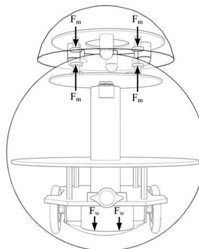
Figure. 8 Model illustration of magnetic balancing unit of CE-R1
