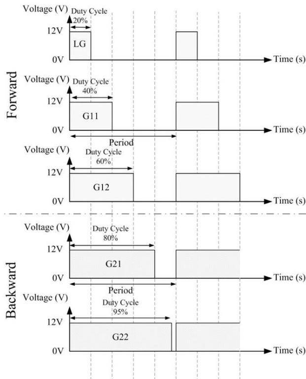
Figure. 10 Pulse width modulation for tuning up a series of CE-R1 gears
