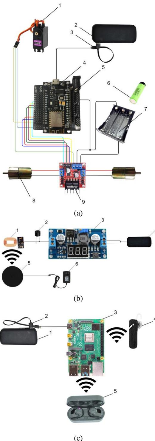
Figure. 4 Components of the spherical magnetic robot 'CE-R1': (a) board controller for controlling the head and body of robot (b) wireless charger and (c) voice recognition
