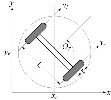
Figure. 3 Geometrical structure of differential drive, where  $\mathbf{q} = [x_r, y_r, \theta_r]^T \in \mathbb{R}^3$
