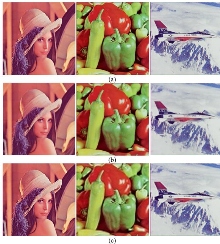
Figure. 17 (a) Original images, (b) fuzzy-BTC with GR results [27], and (c) Proposed QCA-IEGREC results
