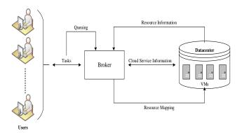
Figure. 1 Broker assisted cloud design
