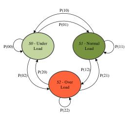
Figure. 3 Load balancing by Markov chain
