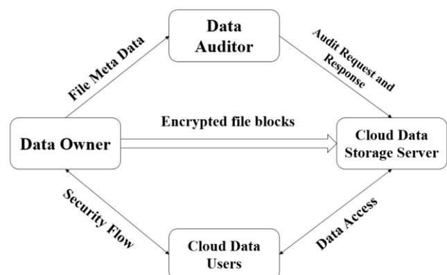
Figure. 1 The system architecture of proposed IRSAC method for dynamic and secure public auditing in cloud
