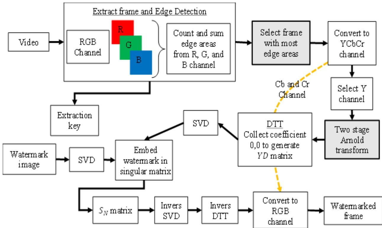
Figure. 3 Visualization of proposed watermark embedding
