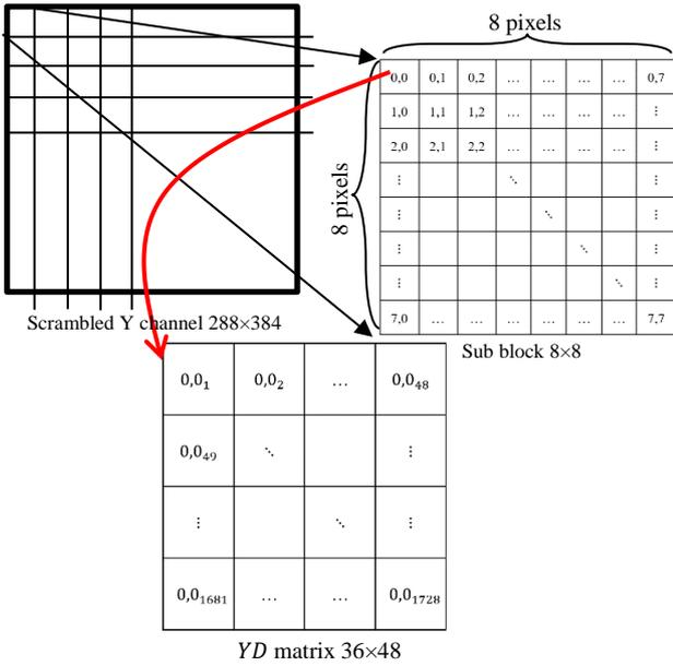
Figure. 2 Illustration of generation  $YD$  matrix
