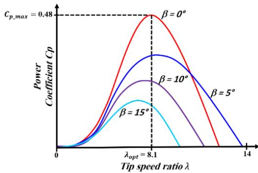
Figure. 1 Power coefficient in terms of ( $\lambda$ ) and ( $\beta$ )
