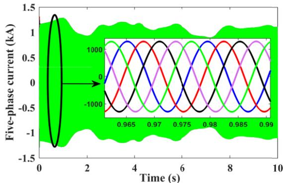
Figure. 14 Generator five-phase current
