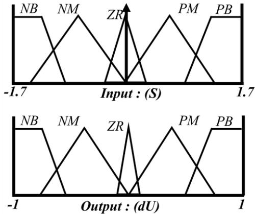
Figure. 3 Membership functions of FL input & output
