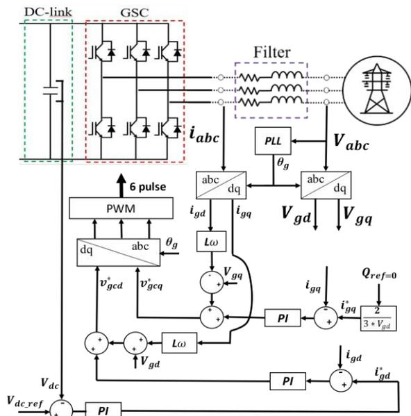
Figure. 6 Grid side converter control
