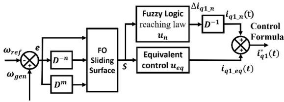
Figure. 2 Proposed fuzzy sliding mode control scheme for speed loop
