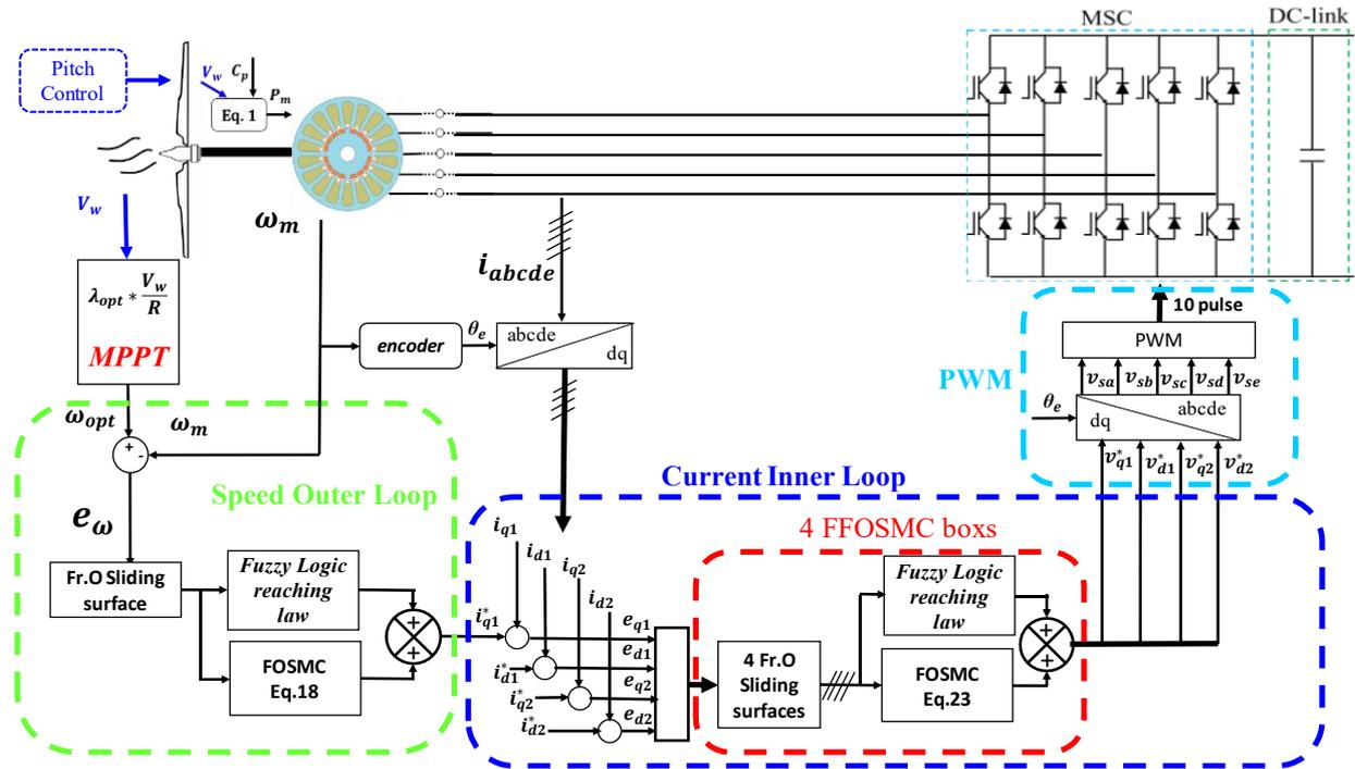
Figure. 5 Scheme of the overall control system
