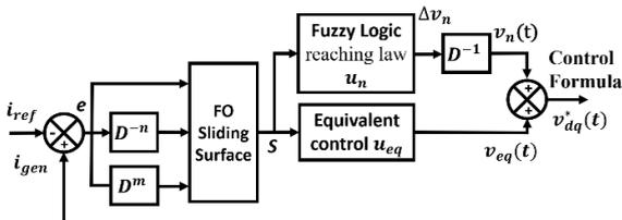
Figure.4 Proposed fuzzy sliding mode Control scheme for current loop
