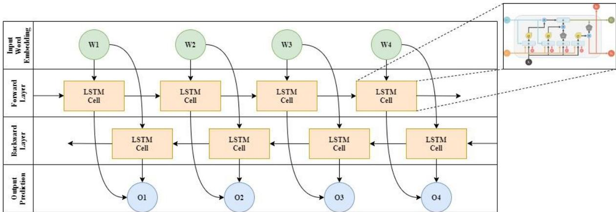
Figure. 2 Bidirectional LSTM architecture
