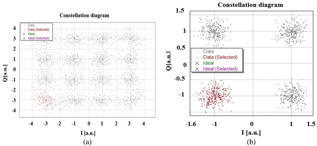
Figure. 10 constellation diagram of received signal after DSP: (a) QPSK and (b)16-QAM
