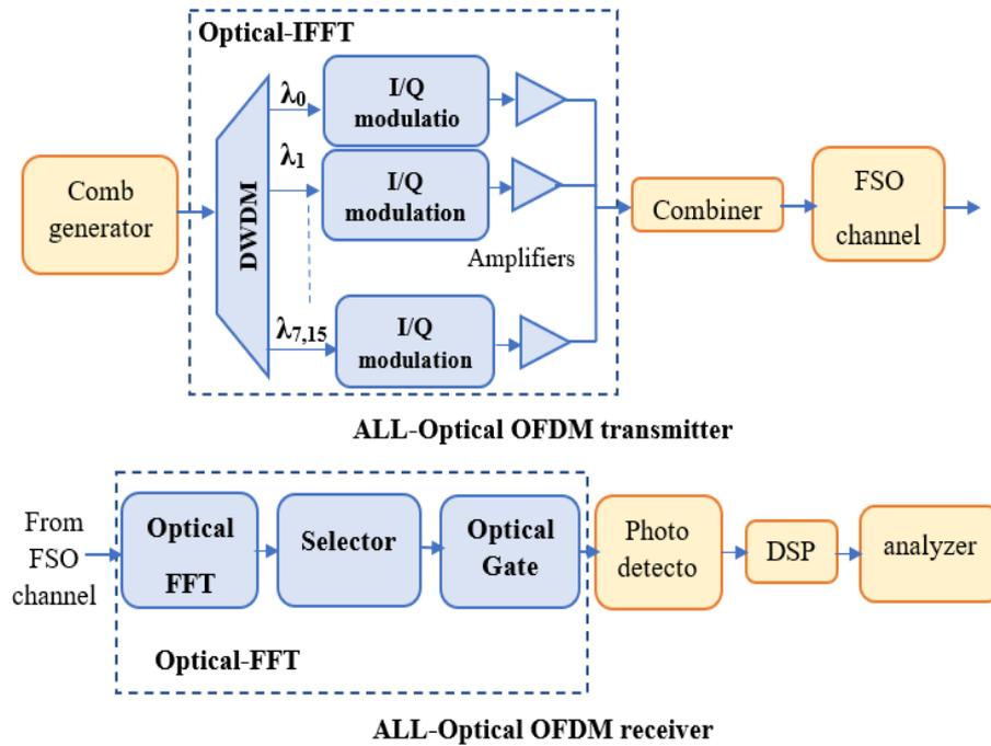
Figure. 3 Li-Fi based AO-OFDM system architecture
