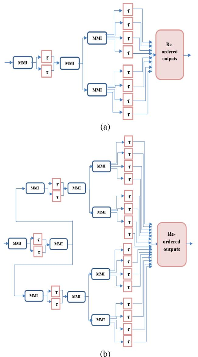
Figure. 5 Optical FFT architecture at receiver side
