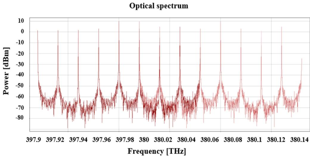
Figure. 6 Frequency spectrum of OFCG with frequency spacing 20GHz
