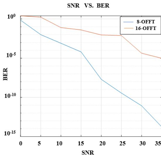
Figure. 11 SNR vs. BER for 8-OFFT and 16-OFFT with QPSK
