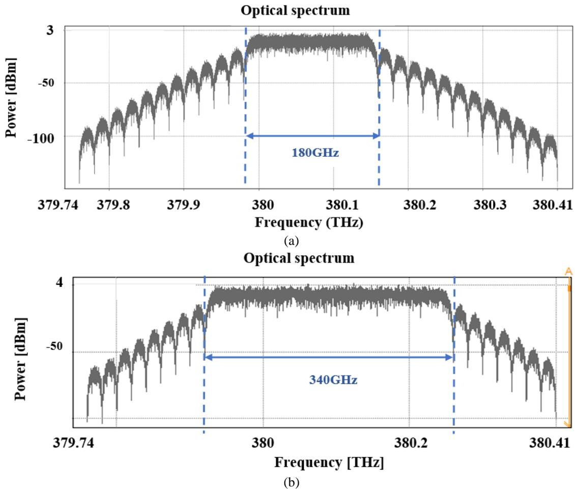
Figure. 8 Frequency spectrum of AO-OFDM signal: (a) 8 channel and (b)16 channel
