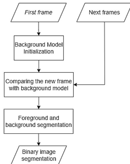
Figure. 9 Segmentation process
