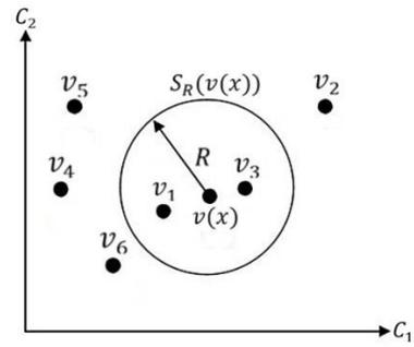
Figure. 8 Pixel classification using a circular area  $S_R(v(x))$  in a two-dimensional euclidean color space  $(C_1, C_2)$
