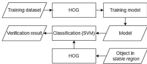
Figure. 13 Vehicle Verification process
