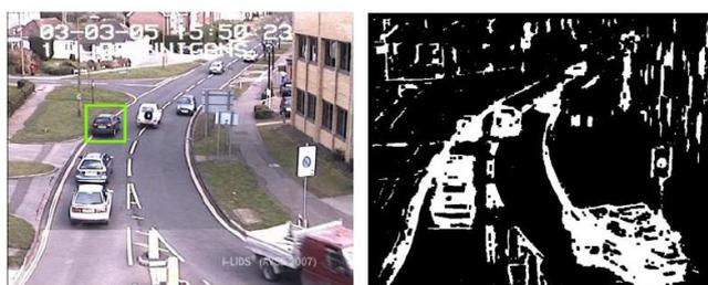
Figure. 19 Example of the effect of camera vibration on segmentation results
