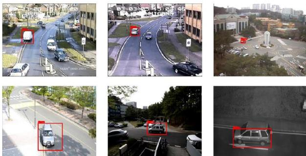
Figure. 18 Example of detection results
