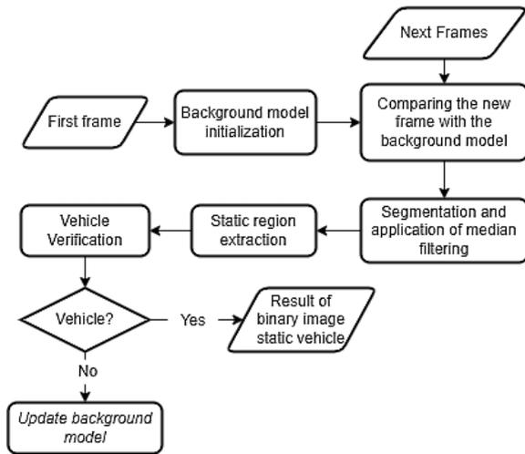
Figure. 1 I-ViBe for detecting illegal parking
