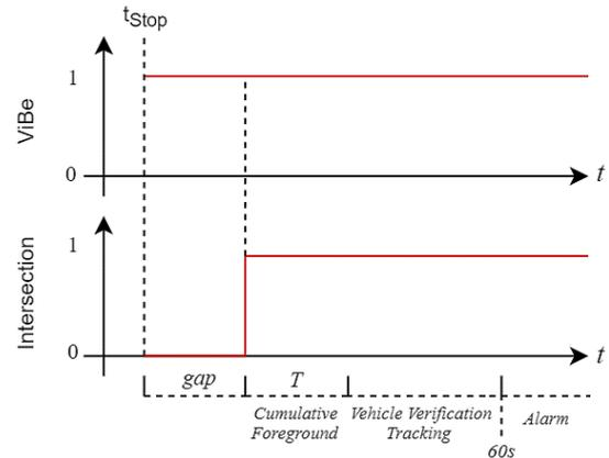
Figure. 14 Overall process flow until the alarm is triggered
