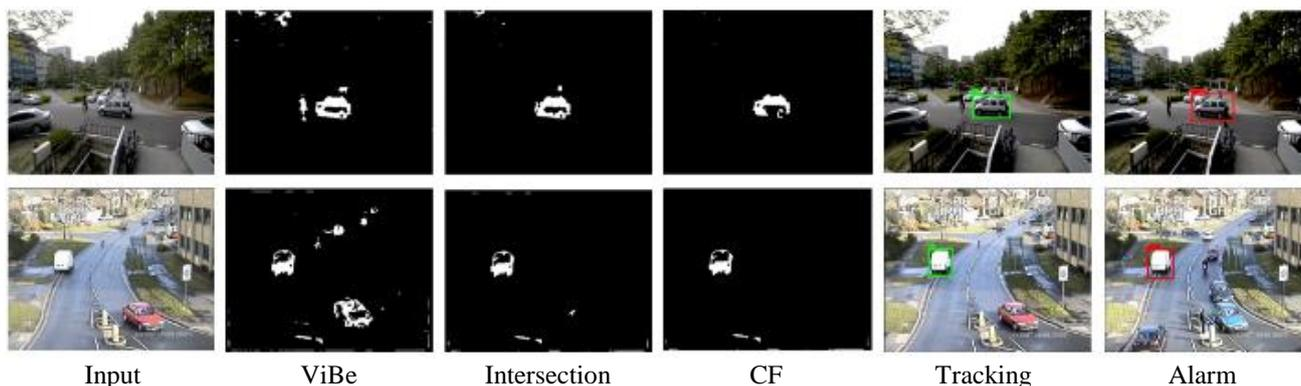
Figure. 20 Examples of the integration in each process
