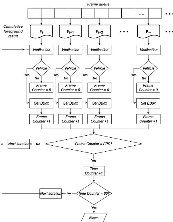
Figure. 15 Tracking process
