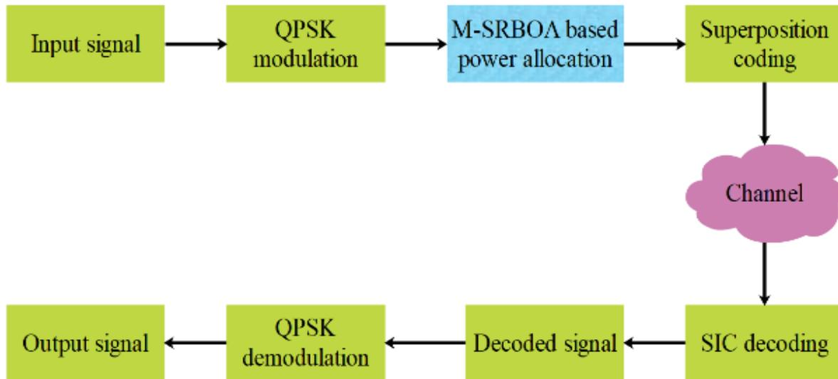
Figure. 1 Block diagram of the M-SRBOA method
