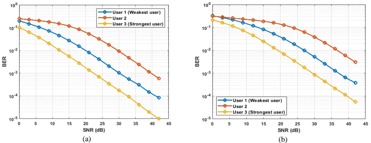
Figure. 3 Analysis of BER: (a) For  $\sigma_i^2 = 2$  and (b) For  $\sigma_i^2 = 10$
