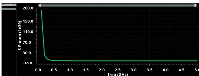
Figure. 9 Stability factor plot of 3 stage LNA
