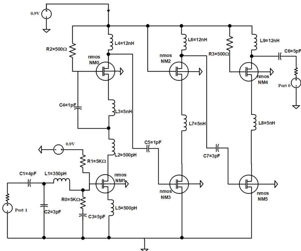
Figure. 1 Schematic diagram of the 3 stage LNA architecture
