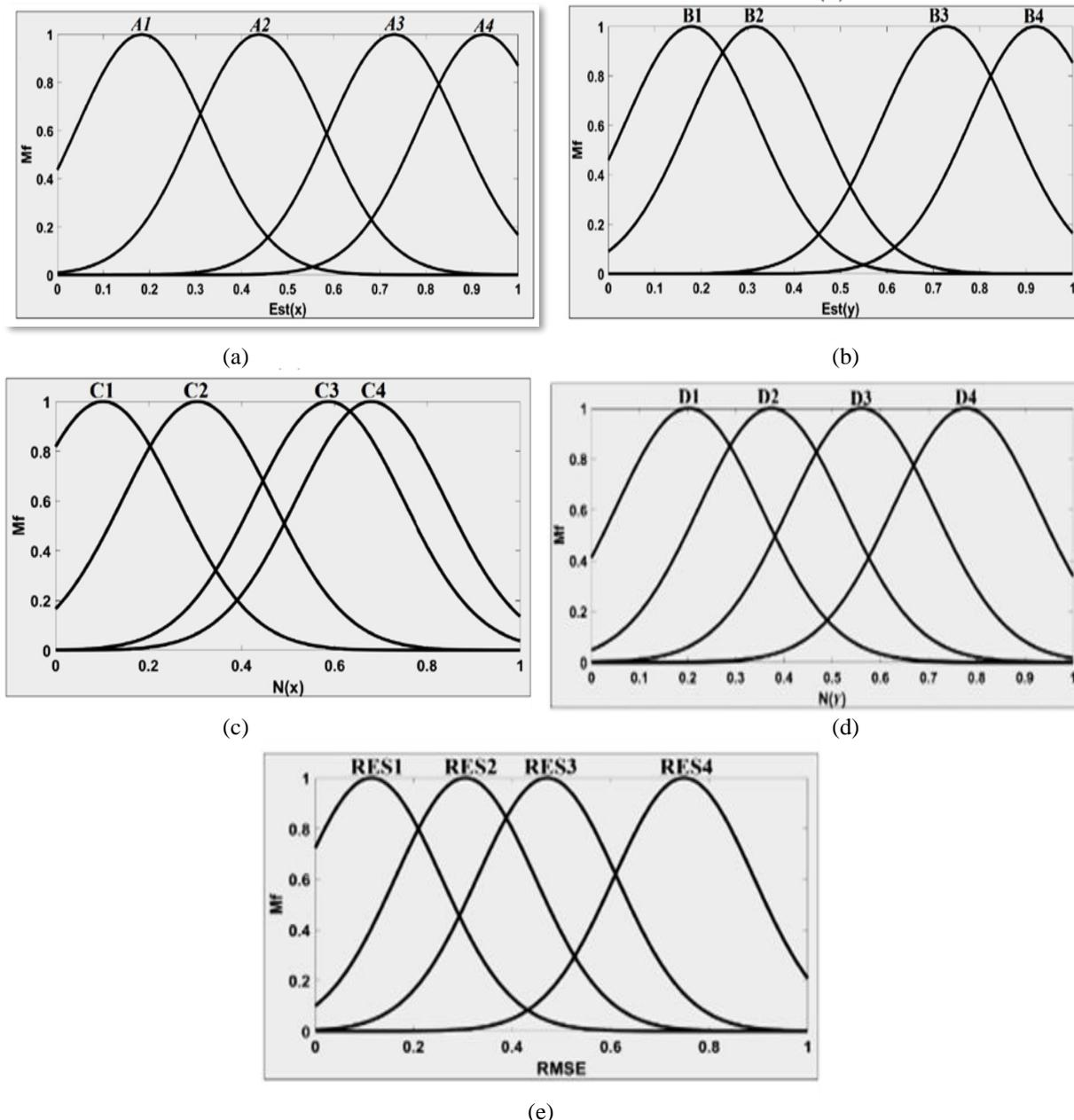
Figure. 3 Gaussian membership functions: (a) estimated x dimension, (b) estimated y dimension, (c) noise in x, (d) noise in y, and (e) root mean square errors
