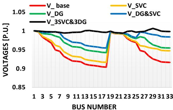
Figure. 6 Improvement of voltage profile of IEEE 33\_bus system
