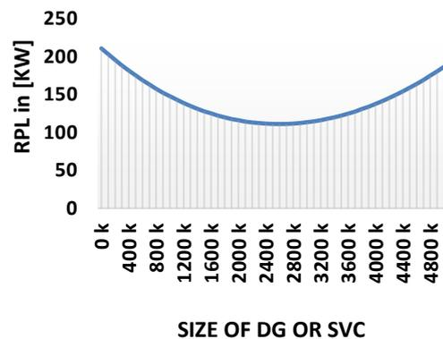
Figure. 3 The relation between real losses and size
