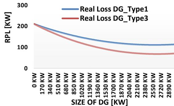
Figure. 7 The Impact of the DG types on the losses in IEEE 33\_bus
