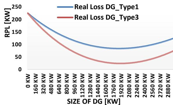
Figure. 10 Impact of DG types on real loss in IEEE 69\_bus system
