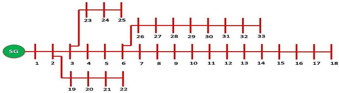
Figure. 5 IEEE 33\_bus test system
