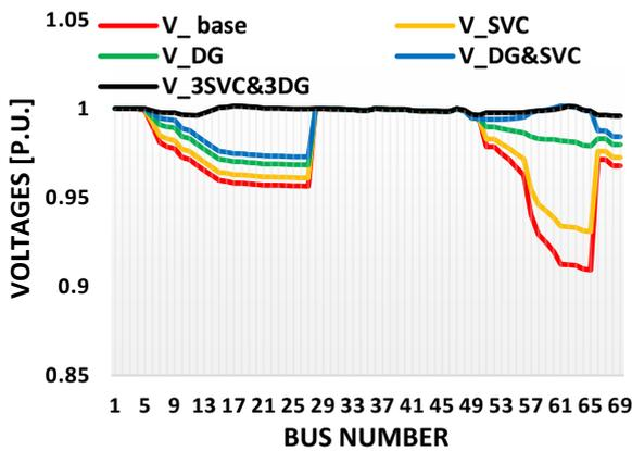
Figure. 9 Voltage profile of four cases for IEEE 69\_bus test system
