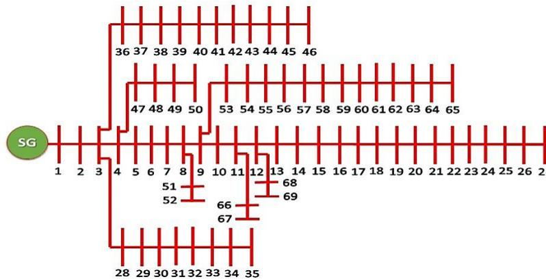
Figure. 8 IEEE 69\_bus test system
