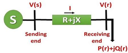
Figure. 2 Equivalent circuit of RDS
