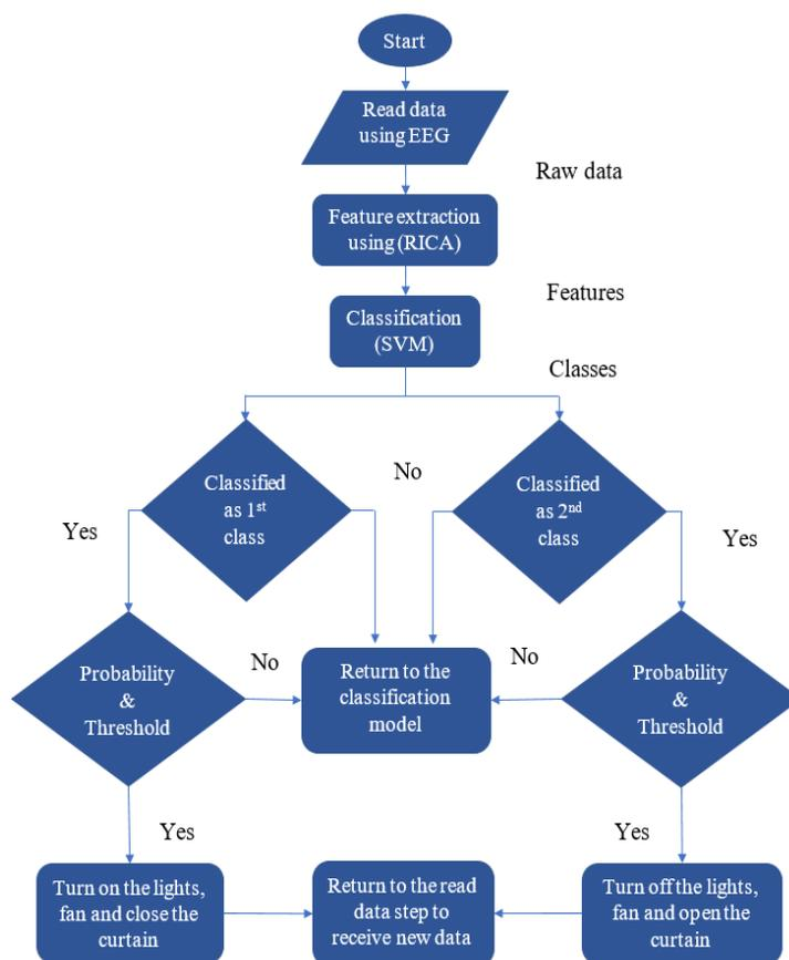
Figure. 3 Flow chart of the work
