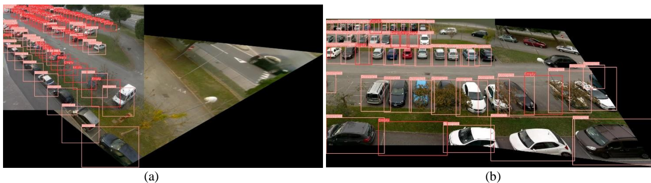
Figure. 5 The result of parking slot occupancy detection from two overlapping cameras on: (a) stitched image of Camera 1 and 2 and (b) stitched image of Camera 3 and 4
