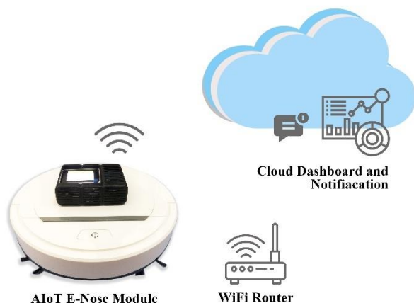
Figure. 1 AIoT electronic nose integrated in vacuum cleaner robot
