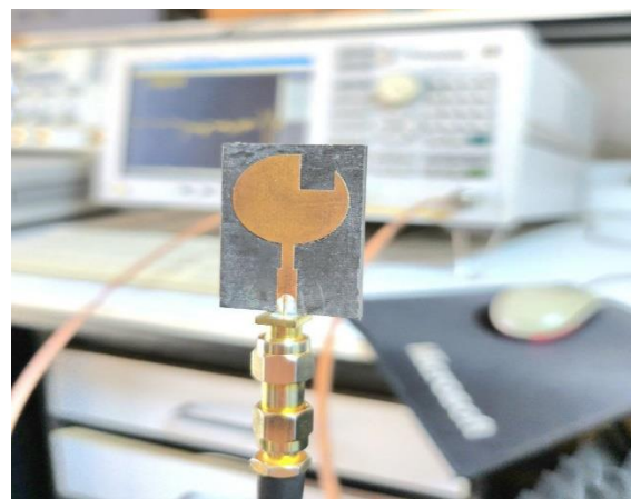
Figure. 13 The implemented Antenna: (a) Patch Layer, (b) Ground Layer, and (c) VNA measurement setup
