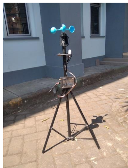
Figure. 5 IoT device for weather monitoring
