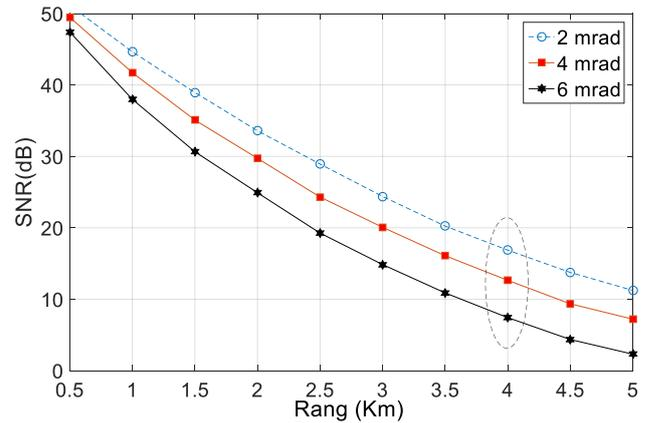
Figure. 5 SNR in relation to link range under different beam divergence situations.
