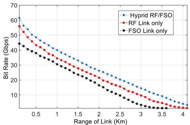
Figure. 7 The relationship between the proposed RF/F
