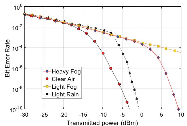
Figure 8 The BER versus variation of transmitted power for the hybrid RF/FSO under different weather conditions.
