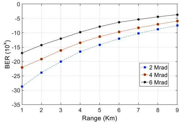
Figure. 6 BER in relation to link range under different beam divergence situations.
