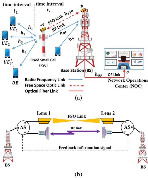
Figure. 2 Proposed model of RF/FSO – OF: (a) end-to-end with multi-hop FSC stations; (b) with Backhaul Selection Algorithm (BSA).
