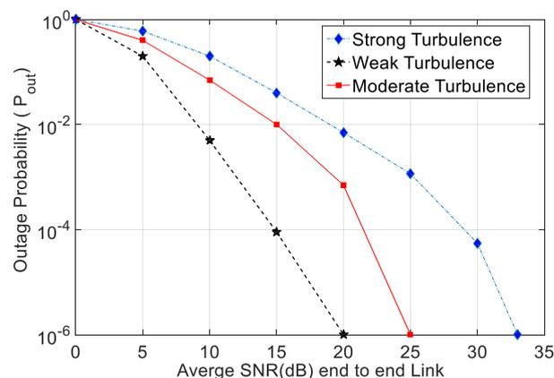
Figure. 11 The relationship of outage probability vs SNR of the proposed RF/FSO-OF system under different atmospheric turbulence conditions.
