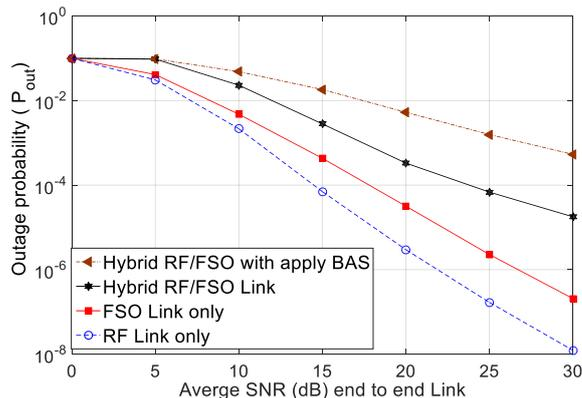
Figure. 9 The relationship of outage probability vs SNR for three scenarios RF/FSO, FSO, and RF links before and after applying BSA.
