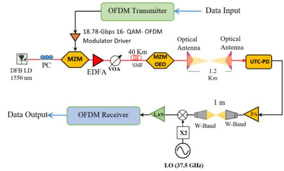
Figure. 3 Framework for Integrated Fiber and Free-Space Optical Communication Systems
