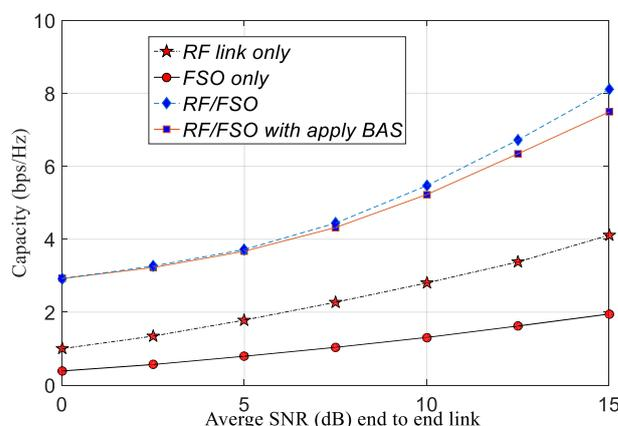
Figure. 10 The relationship between the link capacity and the average end-to-end SNR for RF/FSO, FSO, and RF links before and after applying BSA.
