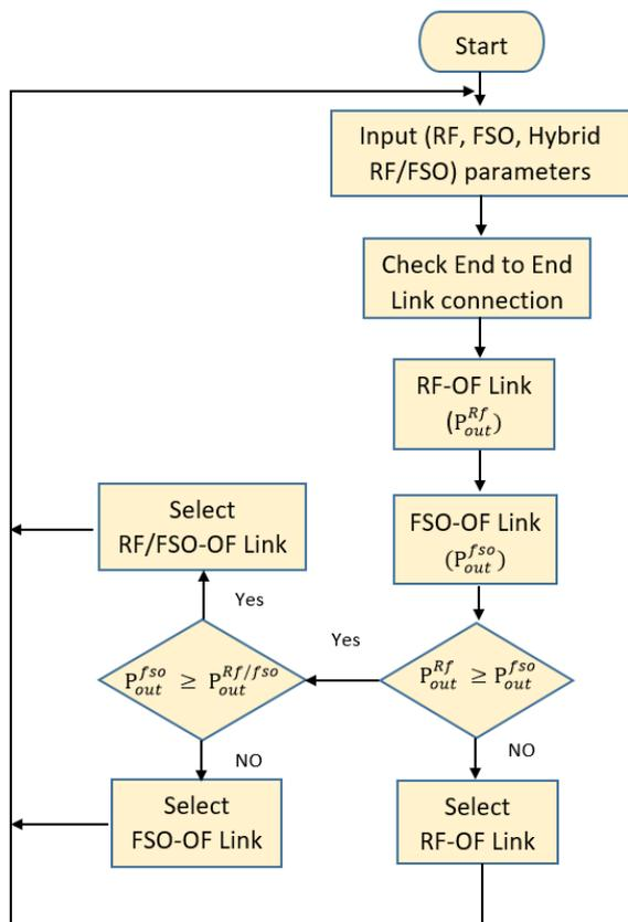
Figure. 4 The Suggested Backhaul Selection Algorithm (BSA) to elect the optimal backhaul link.
