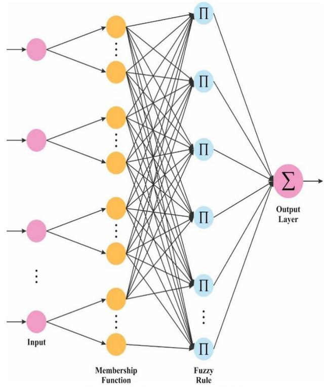
Figure. 2 Structure of DFNN
