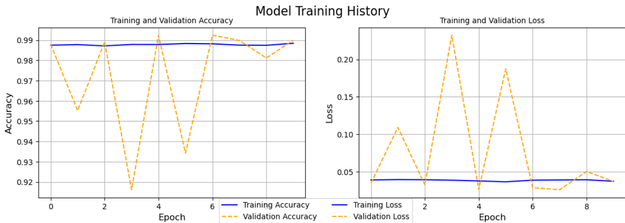
Figure. 11 Training and validation accuracy/loss for the proposed 1D-CNN in binary classification scenario
